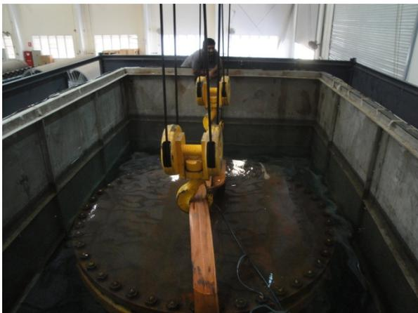
Long-term testing of Flange-Connection PE100, ID1900, PN6
