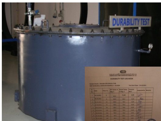
Pic 8: durability test acc. DIN EN ISO 14830 (vacuum test at 80°C)
