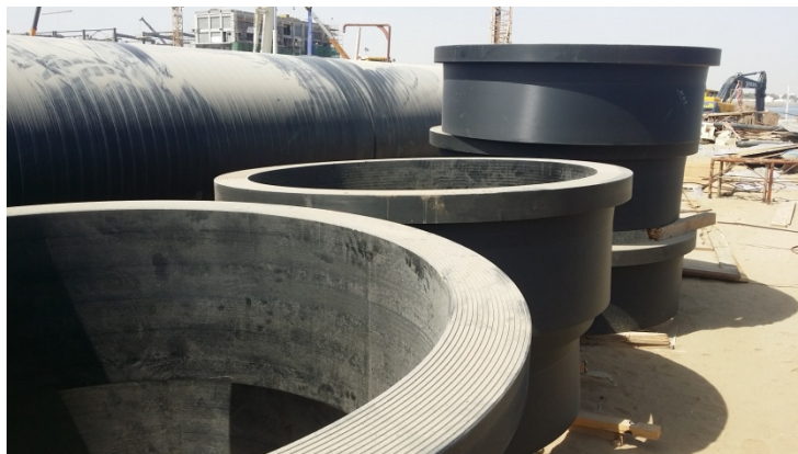
Stub-ends, ID1700, PE 100, PN6, for sea-outfall-project
