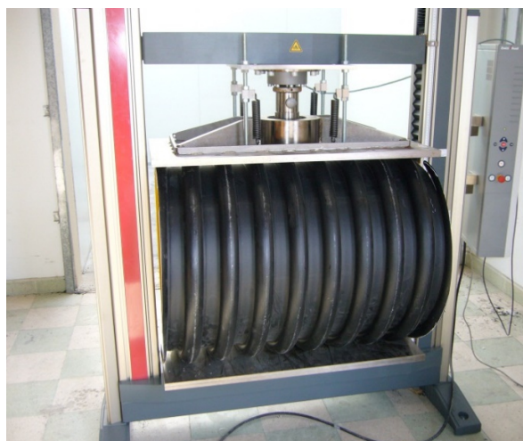
Pic.1 and 2: Ring stiffness test process acc. ISO 9969 and DIN 16961
